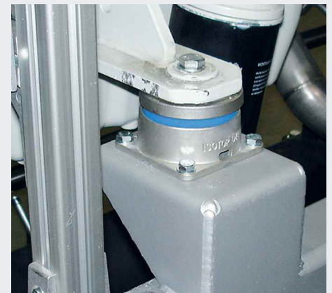
Isotop® DZE bearings for compensating high dynamic forces of very high amplitudes
