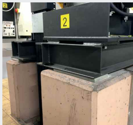
Decoupling of the drive using pre-stressed bearings made from Sylomer®
